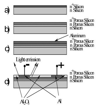
Schematic view of fabrication process and a PS LED structure: a) n-type silicon wafer with  $n^+$ diffused layer; b) after anodization in transition regime, PS is formed both in  $n^+$ - film and in a substrate layer; c) aluminum layer is deposited by magnetron sputtering; d) the final structure after photolithography and sub-sequent aluminum anodization. Light emission at the edge of negative biased pad is evidenced.
