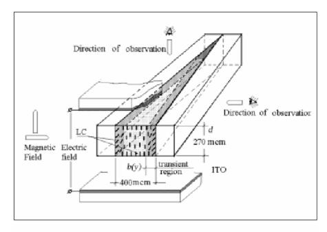
FIGURE: General scheme of the LC cell.
